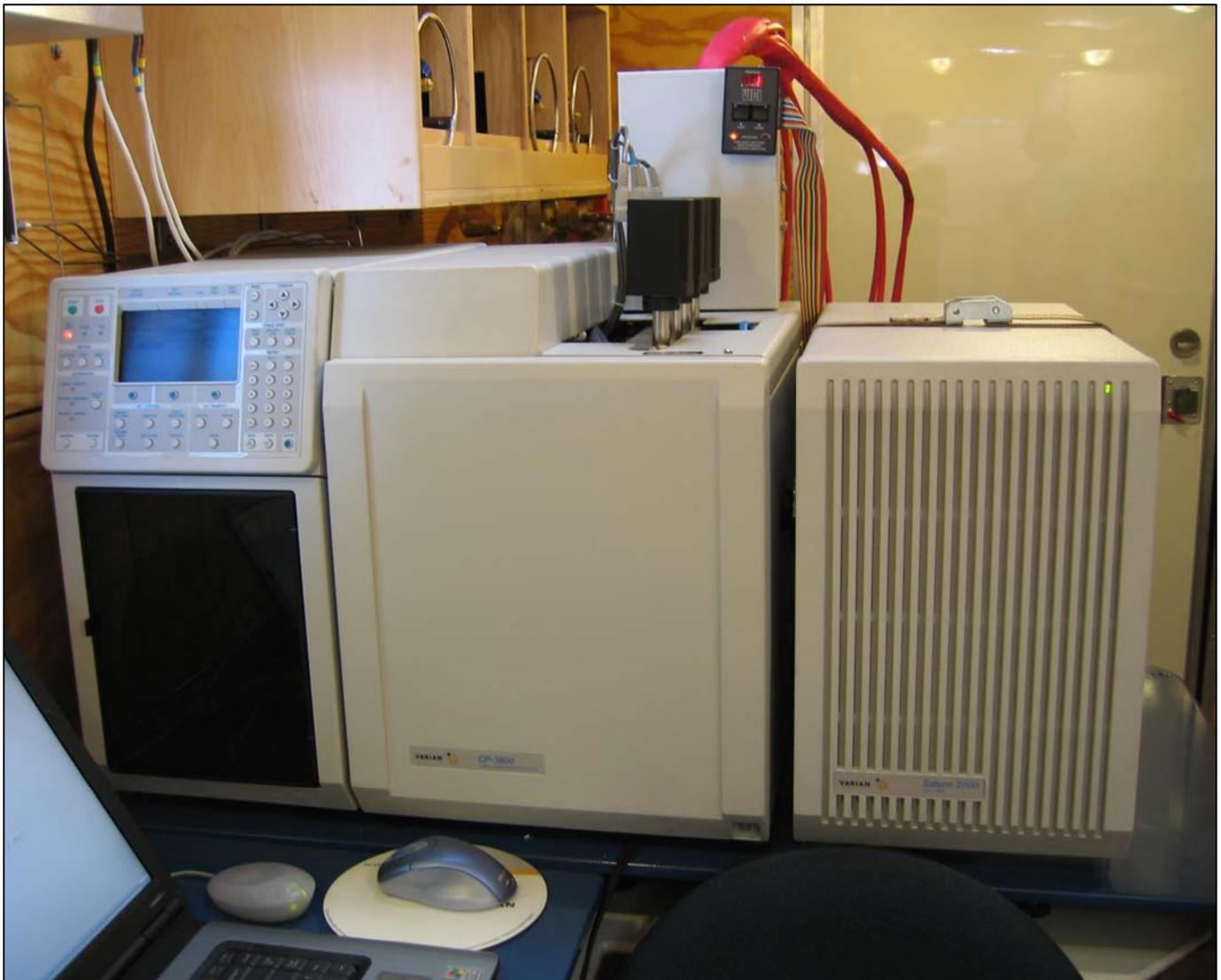
**Multi-detector Trace Toxics System by Lotus Consulting is shown mounted inside a mobile van, with all four detectors fully functional to measure a wide array of toxic compounds in a single sample.**
